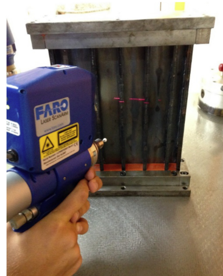
Fig. 4. Imperfection measurements using the laser scanner.
