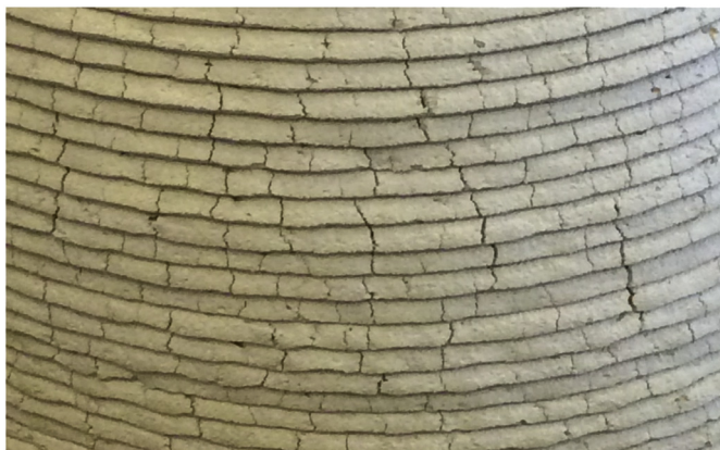
Fig. 1. Excessive shrinkage cracking in an early showcase 3D printing mortar element, as an example of 'bad practice'. (Courtesy G. De Schutter.)
