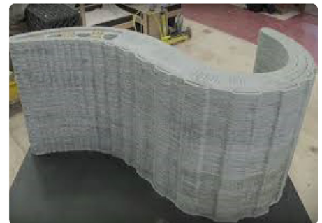
c) a solid geometry, vertically printed component: Loughborough University, UK
