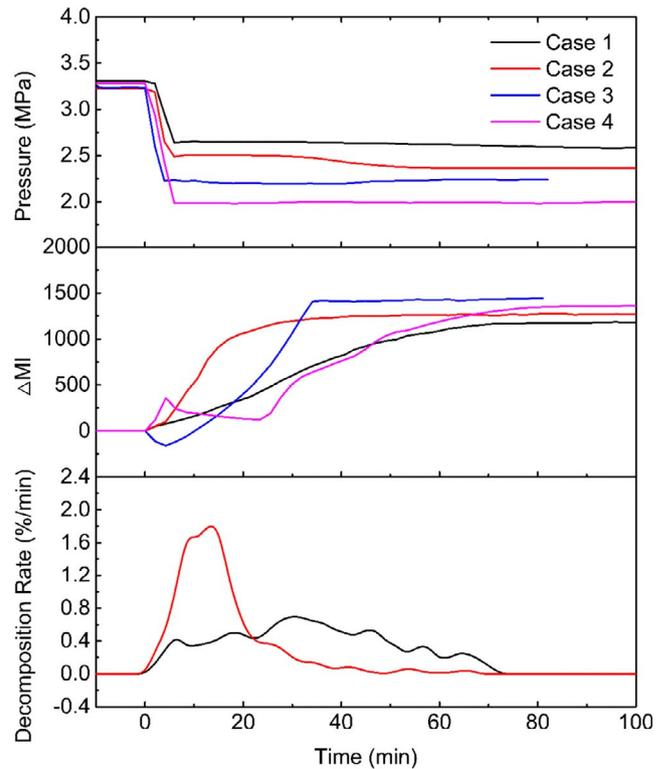
Fig. 2. Vessel pressure (top panel) and MI variation (middle panel) vs. time during the hydrate decomposition process for the sudden depressurization experiments (Cases 1–4). The bottom panel shows the decomposition rates for Cases 1 and 2 calculated using Eq. (2).
