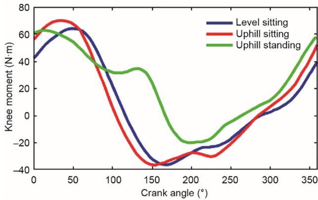
**Fig. 1.** Knee moments corresponding to three cycling conditions: level sitting, uphill sitting, and uphill standing, as adapted from Ref. [4]. The crank angle is measured in the clockwise (CW) direction from the crank top dead center (TDC). The knee-extension moment is positive and the knee-flexion moment is negative.
