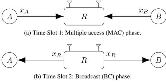
Fig. 1. Two-time-slot two-way relay communication.
