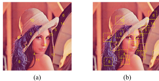
Fig. 2. SIFT feature points: (a) n distinct feature points selected on Lena and (b) extraction of overlapped blocks using n feature points.
