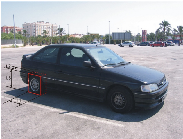
Fig. 1. Parallelepipedic reference surface defined for the A-CPX test.
