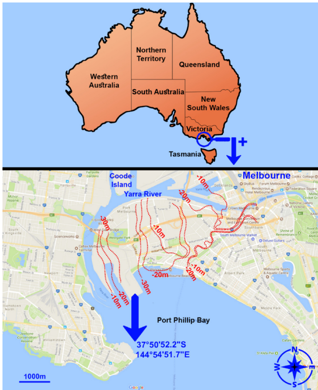
Fig. 1. Contour lines for the base of CIS in the area of interest between the northern shoreline of Port Phillip Bay and Coode Island (after Jamali et al. [6]).
