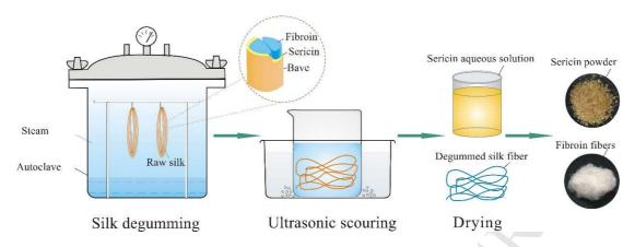
Silk degumming by steam and the recovery of sericin from degumming scouring water.
