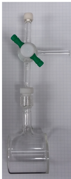
Fig. 1. Photograph of the 2” diameter x 2” length borosilicate glass test cell with purge and septa ports.
