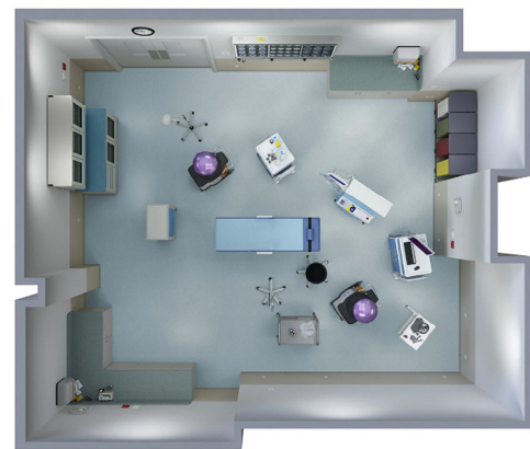
Fig 2. Placement of PX-UV disinfection system for terminal cleaning of operating rooms
