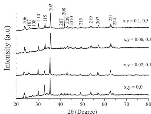
Fig. 2. XRD patterns for  $Ba_{1-x}Dy_xZn_2Fe_{16-y}Mn_yO_{27}$  ( $x = 0, 0.02, 0.06, 0.1$  and  $y = 0, 0.1, 0.3, 0.5$ ) W-type hexagonal ferrites sintered at 1000 °C.
