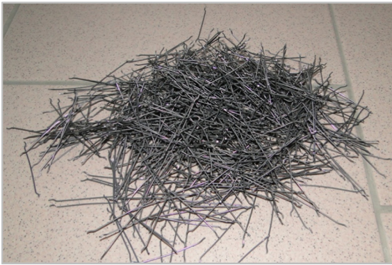
Fig. 1. View of steel fibers used in the research.
