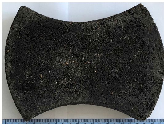
Fig. 3. Typical block paver made in the Cameroon using LDPE and sand.
