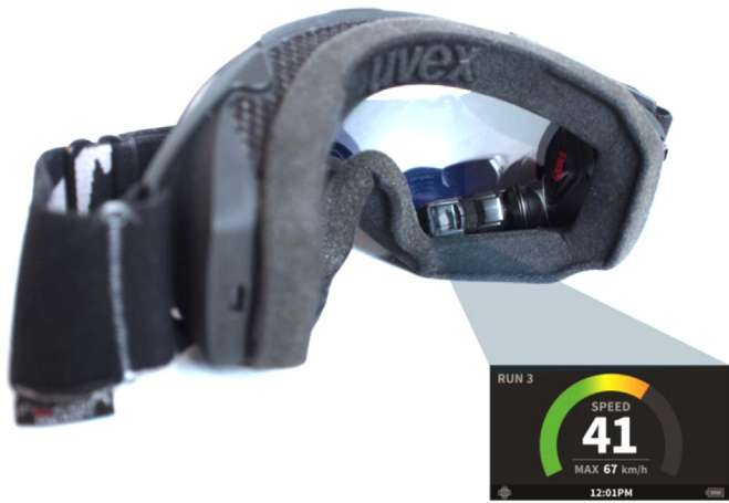
Fig. 1. Recon Instruments MOD Live heads-up-display showing current and maximum skiing speed.
