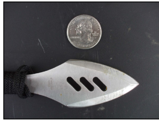
Fig. 1. Double-edge blade used to create lenticular injection port, 1 × 28 mm, by insertion into the trunk. Similar port is created by Bite® injection device with a flat screwdriver-like needle for infusion of trees (Montecchio, 2011).
