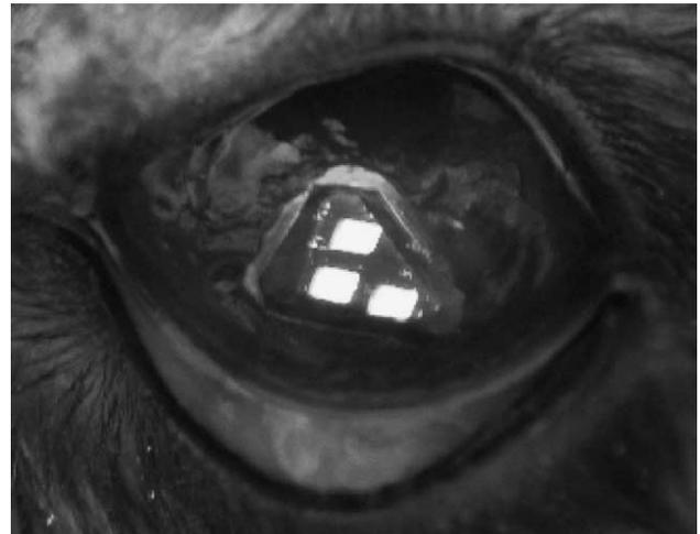
Fig. 1. Fluorescent marker array on the eye of a chinchilla. For this photograph, the eye was illuminated with visible light in addition to UV. Under normal testing conditions, only UV illumination is used, increasing the relative brightness of fluorescent markers.
