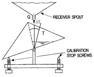
Fig. 1. The tipping-bucket mechanism (after Marsalek, 1981).
