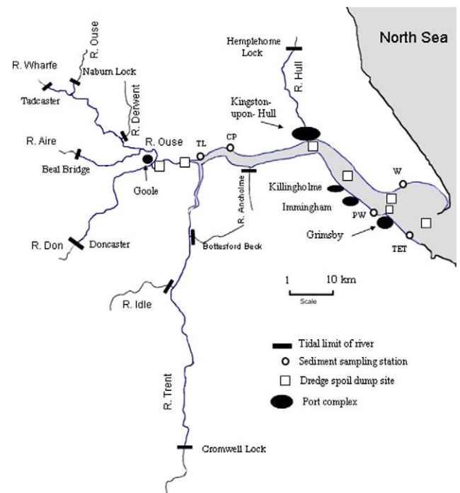
Fig. 2. The Humber estuary and tidal rivers. Tidal limits are indicated by black bars. The rivers all have weirs or locks at their tidal limits, which retard the movement of river sediment downstream into the tidal rivers and estuary. Sediment sampling stations in the estuary are TL (Thornton Lands), CP (Capper Pass), W (Welwick marsh), PW (Pyewipe) and TET (Tetney marsh), sampled as part of the Land–Ocean Interaction Study (LOIS, Leeks and Jarvie, 1998).
