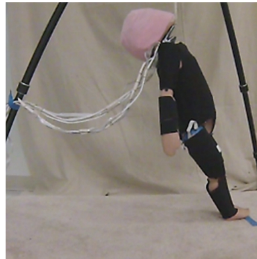
Fig. 1. ATD in an upright initial position (scenario 1) for simulated rearward fall experiments.
