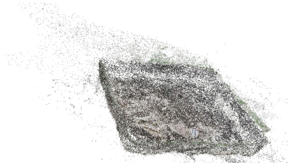
Fig. 1. Sparse point cloud. Note the loose dispersal of points which represent the key points matched throughout the image sequence.
