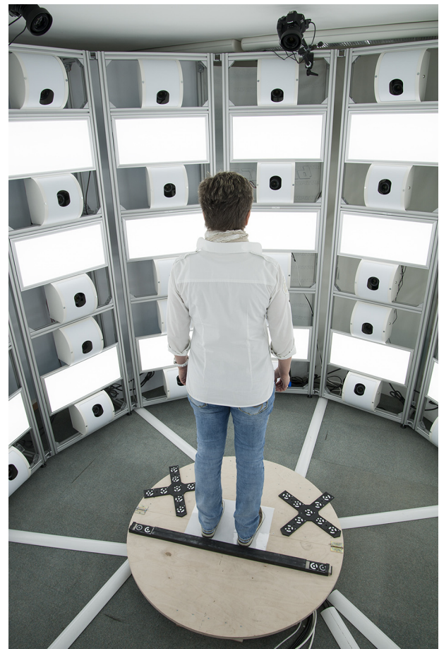
Fig. 2. Person positioned on the platform. The markings on the platform are used for guidance to ensure a uniform procedure. Additionally, the platform is equipped with scale bars.
