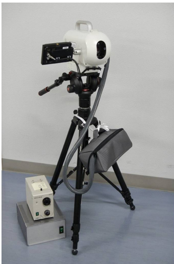
Fig. 1. Snapshot of the portable HSI developed for identifying and detecting untreated latent fingerprints.
