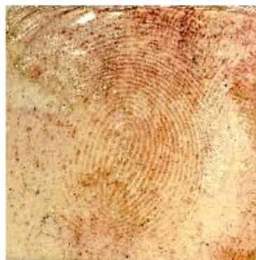
Fig. 1. Fingerprint on print-paper enhanced using Sn modified FDM. (Natural Fingerprint left on paper for 10 days).
