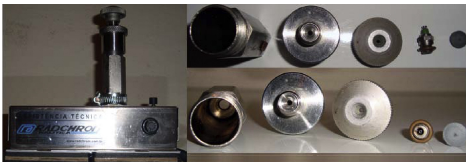
Fig. 1. Burner apparatus used to mimic the burning of stones.
