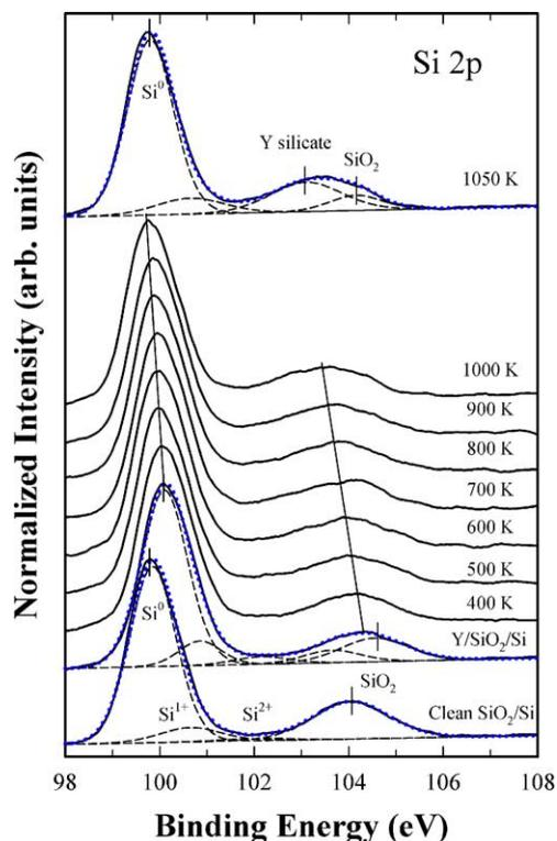
Fig. 1. Si 2p core-level photoelectron spectra obtained from the clean, Y-covered and subsequently annealed SiO<sub>2</sub>/Si(1 0 0) surface.
