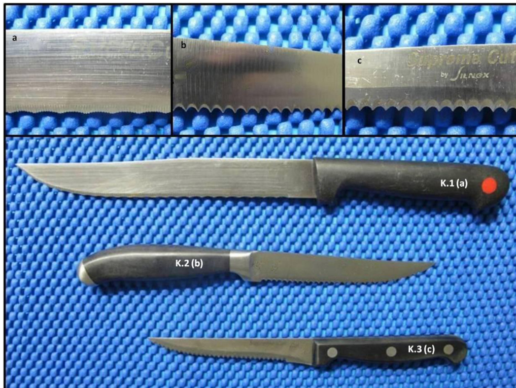
Fig. 1. The three knives used in this study; (a) knife 1, a straight spine, left grounded, mixed pattern finely serrated knife; (b) knife 2, straight spine, right grounded, coarsely serrated knife and (c) knife 3, a straight spine, left grounded, finely serrated knife.
