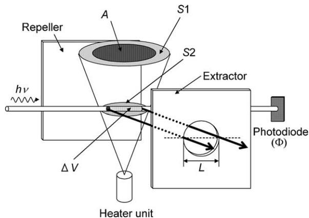
Fig. 2. Illustration indicating the quantities that are required for calculation of the absolute absorption cross section of  $C_{60}$ .  $L$ , reaction length;  $\Delta V$ , ionization volume;  $\Phi$ , photon flux;  $A$ , effective area of the thickness monitor;  $S_1$ , cross section of the molecular beam on the plane including the thickness monitor;  $S_2$ , cross section of the molecular beam on the plane including the ionization region.
