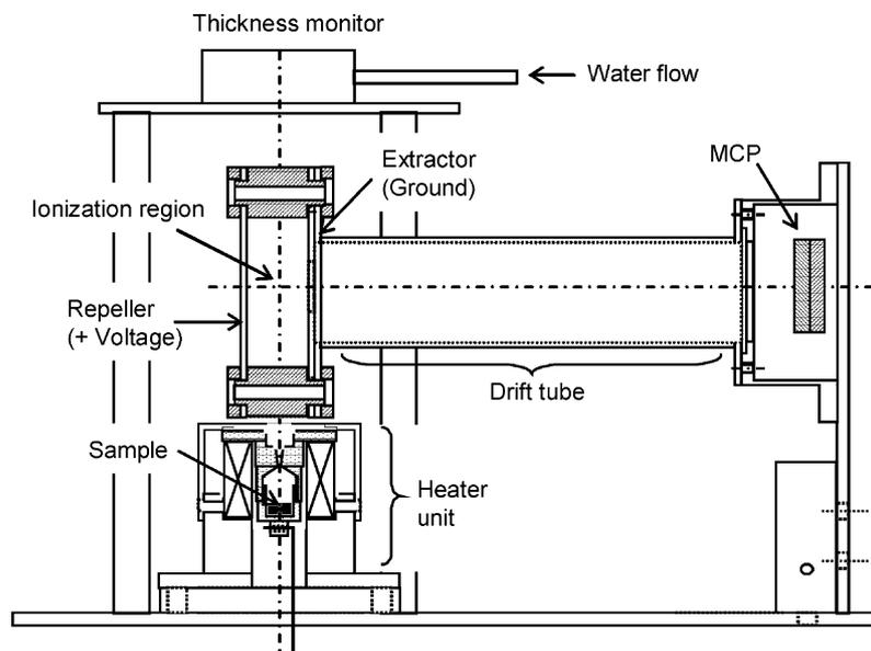
Fig. 1. Schematic diagram of the photoionization mass spectrometer for fullerenes [6].
