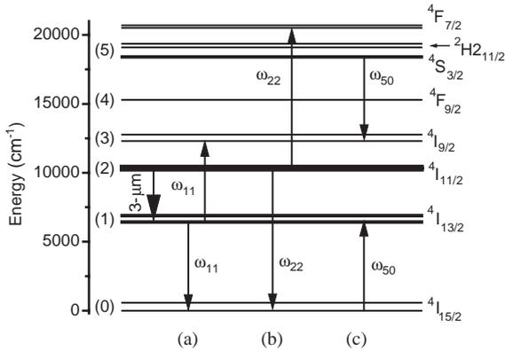
Fig. 1. Energy level scheme of Er<sup>3+</sup> in YAG with the energy transfer processes considered: (a) upconversion from <sup>4</sup>I<sub>13/2</sub>; (b) upconversion from <sup>4</sup>I<sub>11/2</sub> and (c) cross-relaxation from <sup>4</sup>S<sub>3/2</sub>.
