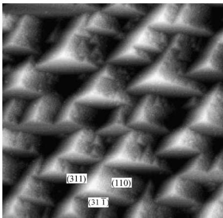
Fig. 1. A  $100\text{ nm} \times 100\text{ nm}$  STM image of the faceted surface prepared by annealing Ir(210) to  $\sim 1800$  K in  $1 \times 10^{-7}$  Torr oxygen background. The vertical scale is  $\sim 2.8$  nm.  $V_g = 100$  mV,  $I = 10$  pA.
