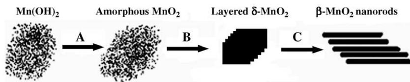
Fig. 1. Schematic representation of the synthesis process of  $\beta$ - $\text{MnO}_2$  nanorods.
