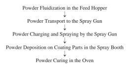
During the operation, paint powder particles for coating are first fluidized and mixed with air in the fluidized bed hopper. These particles are pneumatically carried through a Download English Version:
