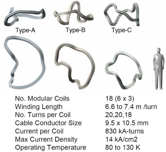
Fig. 2. Modular coil geometry and parameters.
