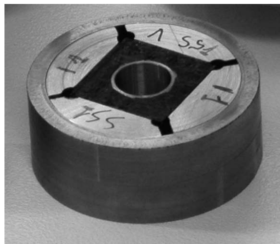
Fig. 1. Picture of the compressive rig with the CFC tile in the center.
