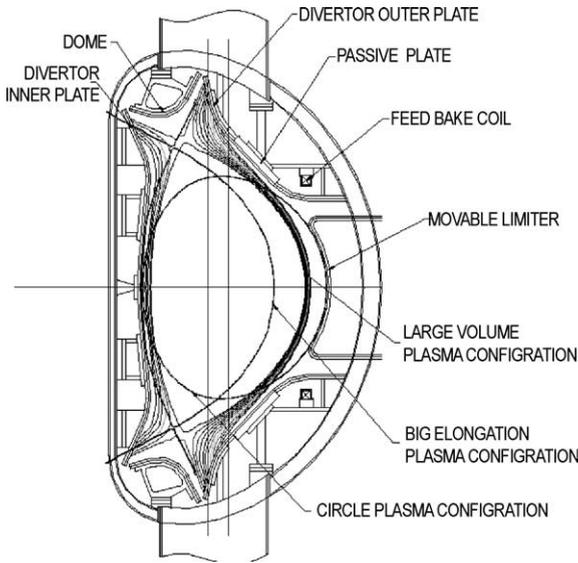
Fig. 1. Elevation view of EAST PFCs.
