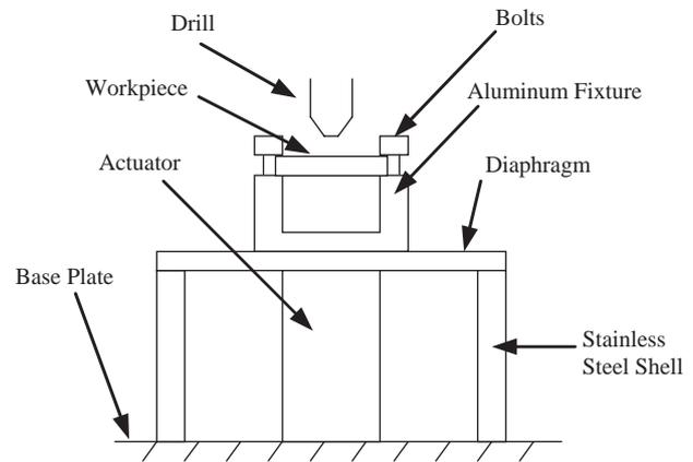
Fig. 1. Cross section of the workpiece holder.
