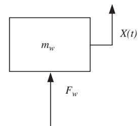
Fig. 2. Free body diagram of the combined mass.
