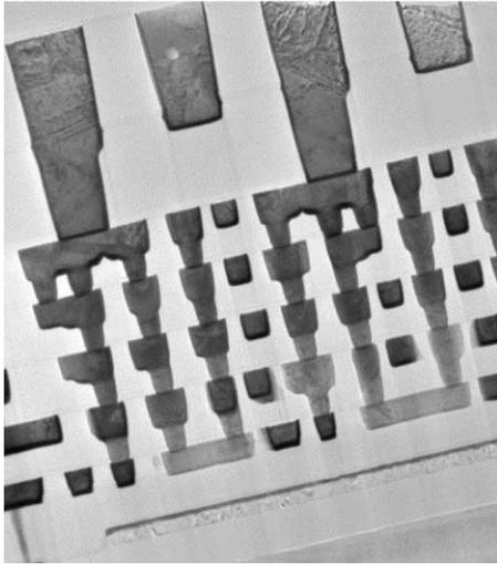
Fig. 1. TEM cross-section of a six-level metal circuit made with low- $k$  dielectric.
