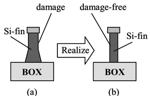
Fig. 1. Comparison between (a) bell-shaped Si-fin by RIE and (b) the proposed ideal rectangular cross-section Si-fin by the orientation-dependent wet etching
