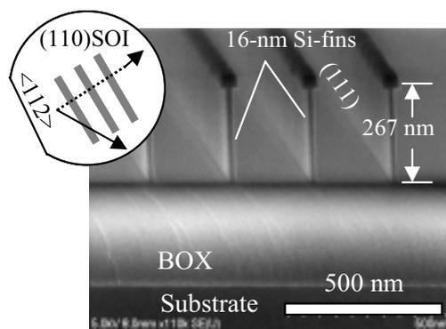
Fig. 3. SEM image of the fabricated 16-nm-thick Si-fin channels. Insert is the schematic fin-patterns on (110) SOI.
