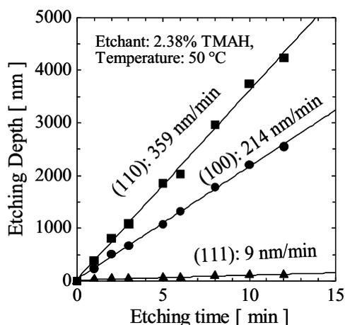
Fig. 2. Etched silicon depth versus etching time in TMAH at 50 °C. The selectivity of (110)/(111) is about 40.
