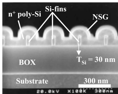
Fig. 4. Cross-sectional SEM image of the fabricated multi-fin channels after gate oxidation,  $n^+$  poly-silicon and NSG deposition. The Si-fin channels show a perfect rectangular cross-section.
