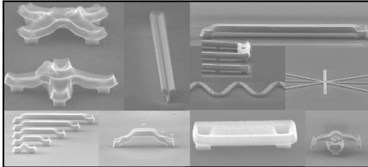
Fig. 1. A gallery of metallic air-bridges fabricated by multiple acceleration voltage electron beam lithography.
