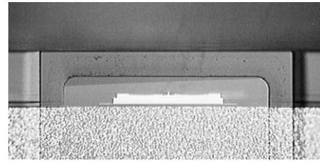
Fig. 2. Optical image of a portion of the air bearing surface used in the study. The darker section near the trailing edge of the air bearing surface resulted from wear.
