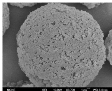
Fig. 1 SEM image of a POROS<sup>®</sup> R1 particle.
