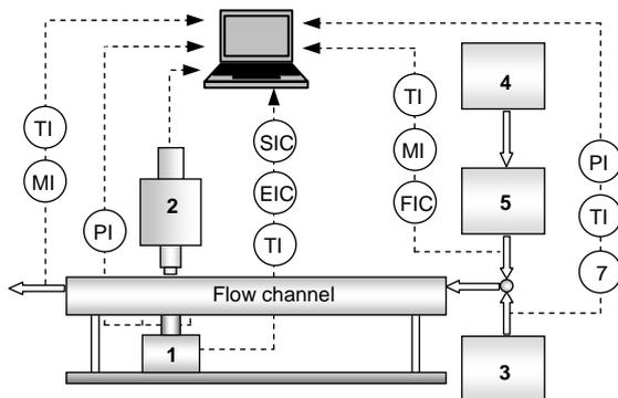
Fig. 2 Experimental set-up: 1 oscillation system with attached substrate; 2 optical unit with microscope, CCD-camera; 3 compressed-air; 4 laminar flow box; 5 climatic exposure test cabinet and flow channel ( $l \times b \times h$ : 1700 mm  $\times$  40 mm  $\times$  4 mm).
