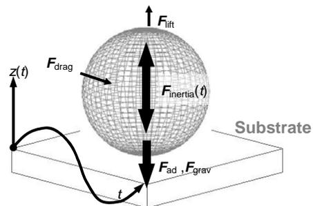
Fig. 3 Forces acting on a single particle exposed to a laminar air flow and adhered to a sinusoidally oscillating substrate.
