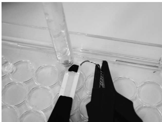
Fig. 1. Experimental set up for the electrochemical measurements in a 50 \mu l drop: the working electrode is a screen-printed graphite one, the counter electrode is a platinum wire and a standard reference electrode Ag/AgCl just touches the 50 \mu l drop.
