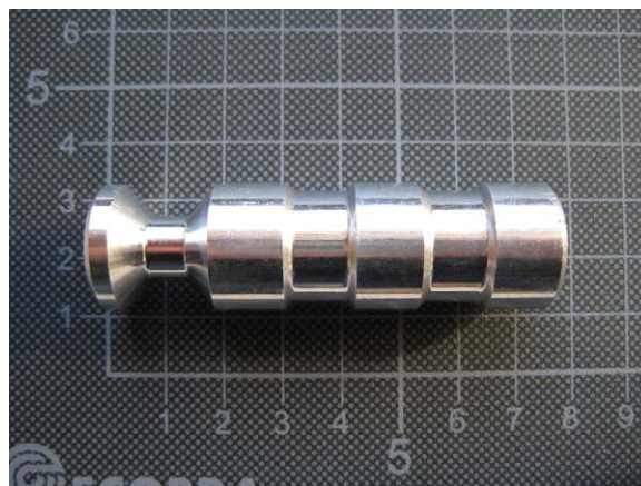
Fig. 3. Aluminium sleeve (outer length 70 mm, outer diameter 20 mm, mass 28 g) cut out of the hard foam dummy. The open right end is imposed on the launcher arm.
