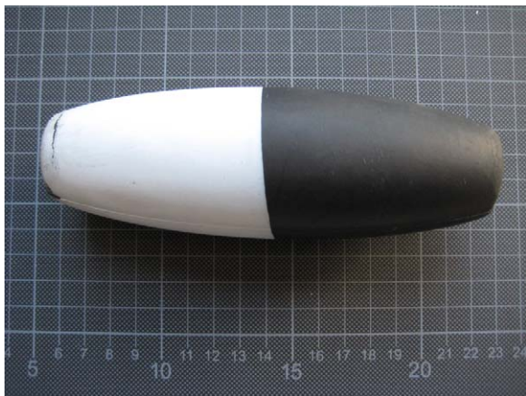
Fig. 2. Flat-nosed hard foam dummy (length 150 mm, front diameter 30 mm, mid diameter 50 mm, mass 130 g). The dummy is imposed on the launcher arm and propelled on a trajectory after discharge.
