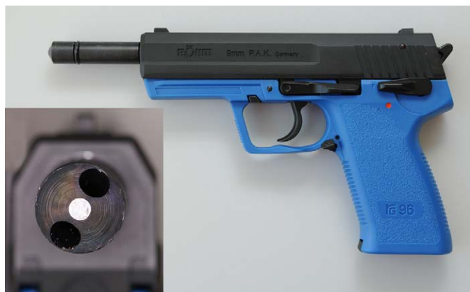
Fig. 1. Roehm Rapid Launcher. The extension tube (launcher arm) is pinned and welded to the barrel imitation and contains an o-ring to prevent gas pressure leakage before the dummy is launched. The muzzle contains two 4 mm boreholes (close-up figure).
