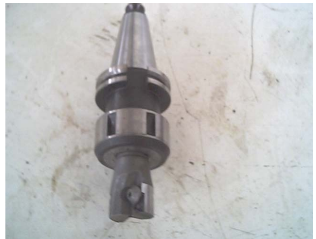
Fig. 1. End milling tool holder used in this study.
