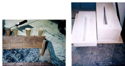
Fig. 2. Pattern and sand mold.
