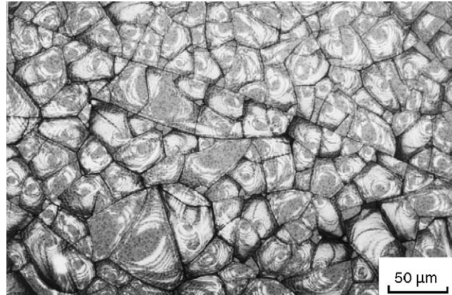
Fig. 2. Optical picture ( 100\times ) of sample surface after radiation. Dark lines and parts indicated cracks/peelings on the surface.
