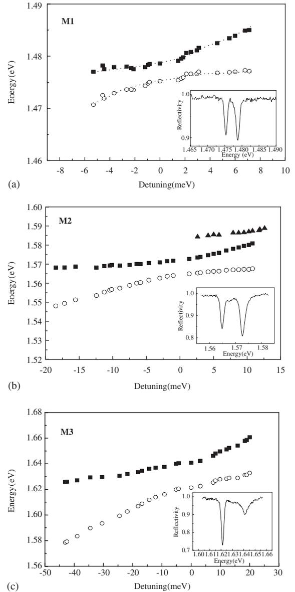
Fig. 1. Polariton energies versus detuning measured in microcavity M1 (a), M2 (b) and M3 (c) at 10 K. The inserts show the reflectivity spectrum at zero detuning.
