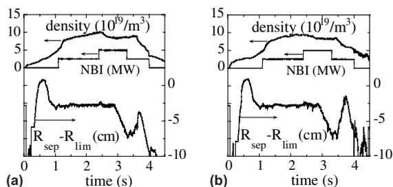
Fig. 2. The temporal behavior of the line averaged density, NBI heating power and  $R_{\text{sep}} - R_{\text{lim}}$ .  $R_{\text{sep}} - R_{\text{lim}}$  means the midplane distance between the separatrix and the test limiter. (a) for #17428. (b) for #17505.
